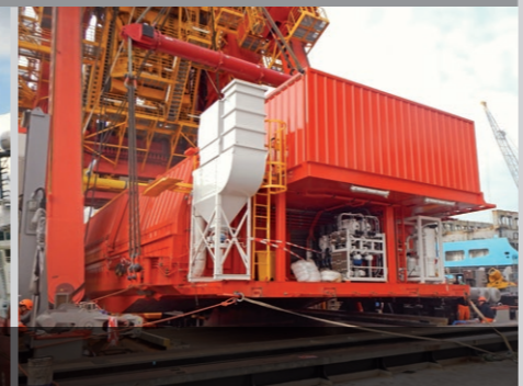
Delivery of land spool base equipment: level winders, reel-drive systems and hydraulic power units.
